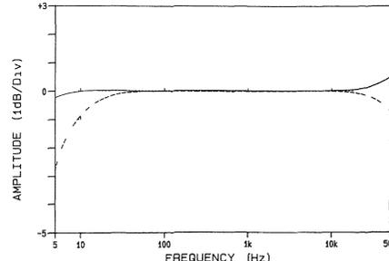
Fig 3 Kenwood L-1000C pre-amp: disc equalization errors, m-m plains line, m-c dashed
