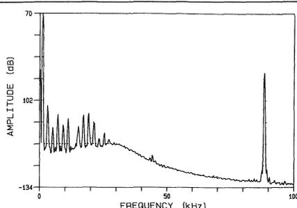
Fig 1 Kenwood L-1000D CD player: spurs associated with 1kHz tone at -70dB
