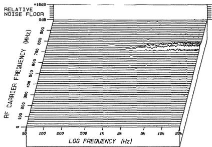
Fig 4 Kenwood L-1000M power amp: 3D display of RF spurs
